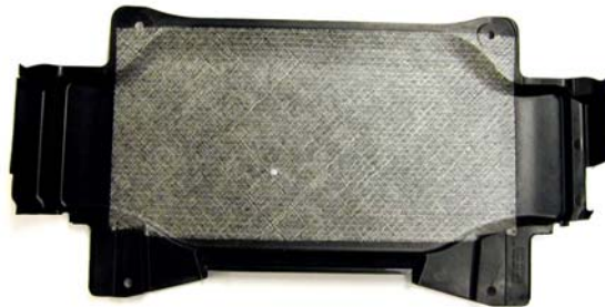
Figure 1. A moulded component in fabric reinforced GMT. The inlay zone consists of combined layers of fabrics and GMT, whereas the flow zone consist of only GMT.
